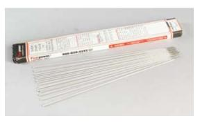
Mild steel type electrode has a special quick start tip. Stable arc and automatic action that makes it easy to use on thin metals requiring low amperage. Features self-cleaning action that works well in all positions. Tensile Strength 60,000 PSI.
